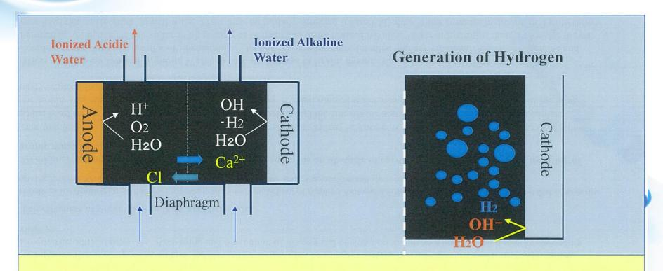
Water is decomposed into hydrogen and hydroxide ion around the electrode when electrolyzing. Hydrogen ion is increased at cathode side and hydroxide ion is increased at the anode side. Receiving electron from electrode, hydrogen ion at the cathode side is changed into hydrogen. It is said that an increment of hydrogen ion at the cathode side causes the change like  $2H++2e \rightarrow H2$ , leading to a rich hydrogen at cathode side.
